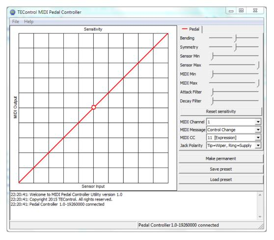
The top left part of the window (graph) shows the current sensitivity curve stored in the controller and can be adjusted with the sliders, drop down menus and buttons located on the right part of the window.
